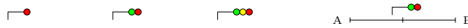
Figure 8.2: Selection of different signals. Left: 1 aspect signal, only shows danger aspect. Centre left: 2 aspect signal, shows danger or proceed aspects. Centre right: 3 aspect signal, shows danger, caution or proceed aspects. Right: signal is only visible when travelling from A to B, also known as facing direction.
