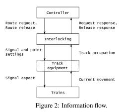
and track circuits detect if there is a train on a track. Finally, *Trains* have a driver who determines their behaviour. For simplicity, we make the (unrealistic) assumption that track equipment reacts instantly and is free of defects.
